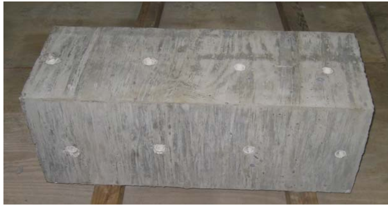
Figure 4.2: Splitting Wedge Test Specimen
