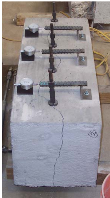
Figure 4.3: Cracked Specimen using Splitting Wedges
