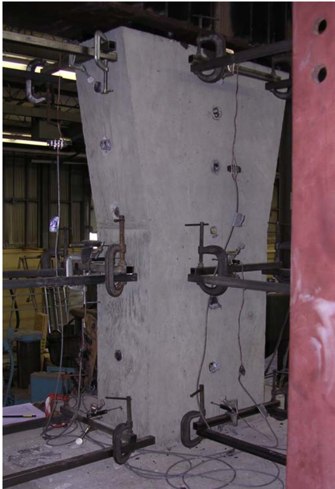
Figure 4.15: Test S2 Linear Potentiometers
