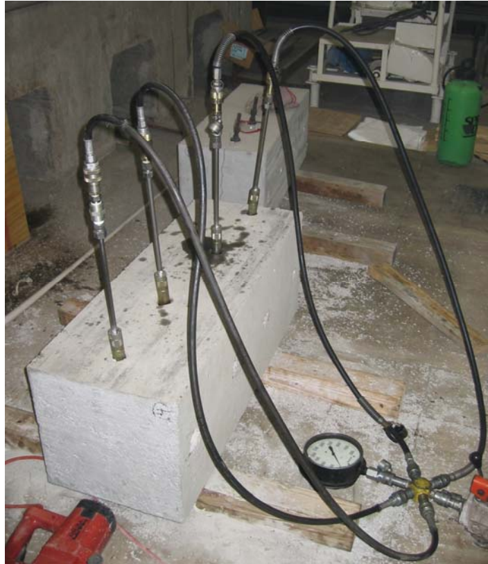
Figure 4.6: Hydraulic Packer Test Setup
